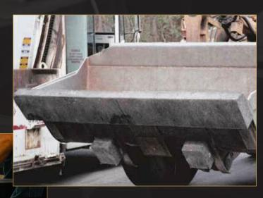
SETCO offers "combo" edges with steel wear guards for added durability.
