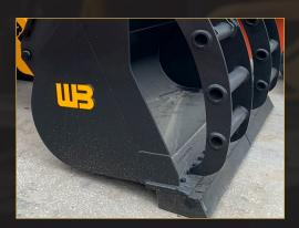
Rubber leveling pads, mounted at the rear, allow the bucket to be operated at the proper angle, minimizing pressure on the cutting edge, increasing longevity.
